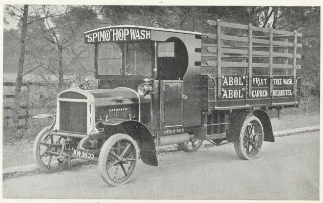
A FARMER'S MULTI-PURPOSE BODY FITTED TO A  $2\frac{1}{2}$ -Ton chassis
