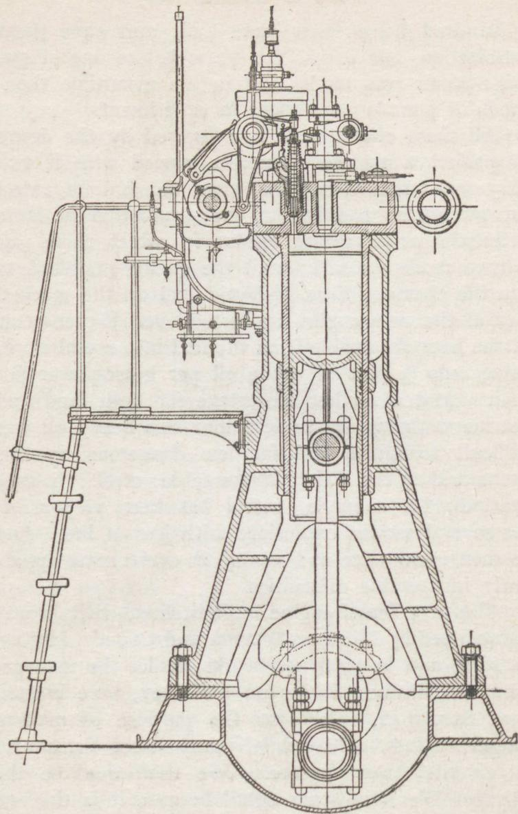
Fig. 132.—Transverse section of Diesel engine
