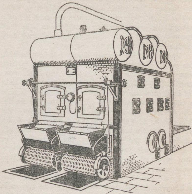
Fig. 39.—Exterior of a Stirling boiler
