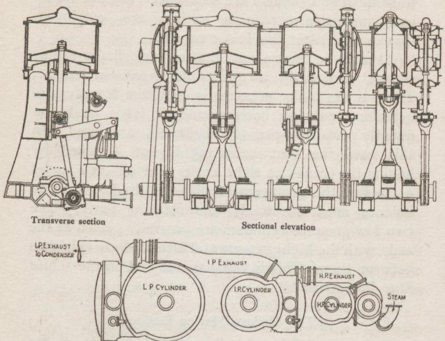
Fig. 156.—Three views of a triple expansion marine engine
