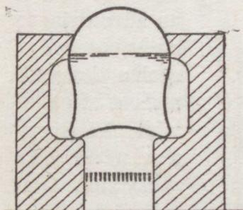
Fig. 25.—Watt's wagon boiler
