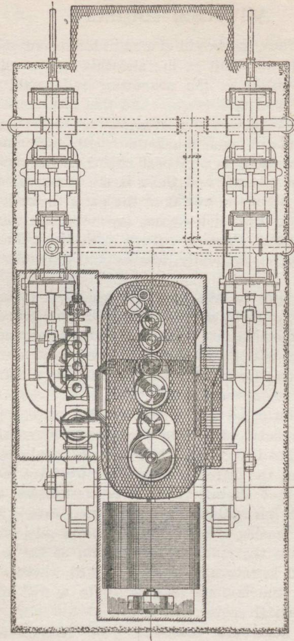
Fig. 81.—Horizontal and vertical engines of equal power drawn to same scale. Plan
