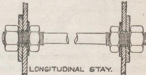
Fig. 21.—How a boiler is strengthened lengthways
