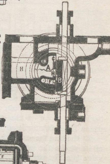
Fig. 164.—Vertical section through valves of Weir pump
