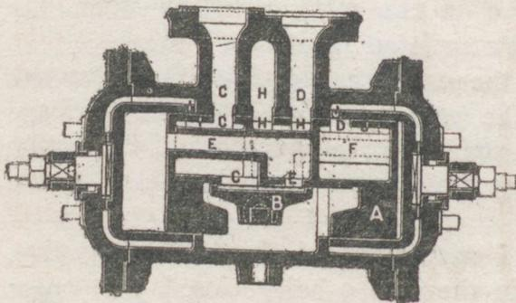
Fig. 163.—Horizontal section through valves of Weir pump
