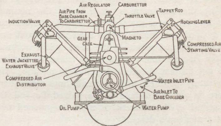
Fig. 130.—Diagram of V type of aeroplane engine
