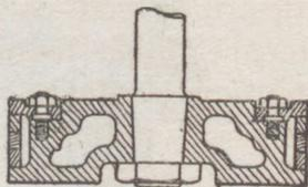
Fig. 60.—Piston with junk ring for large engine
