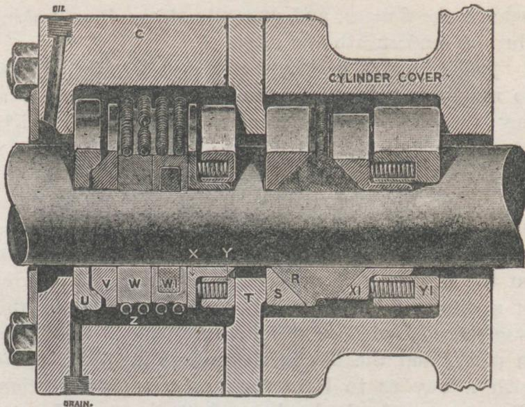
Fig. 63 (a).—Metallic packing for high pressures: Longitudinal section
