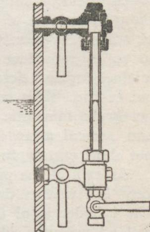
Fig. 4.—Water-gauge in part section
