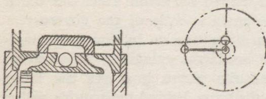
Fig. 9.—Simple slide valve, with no lap and no lead
