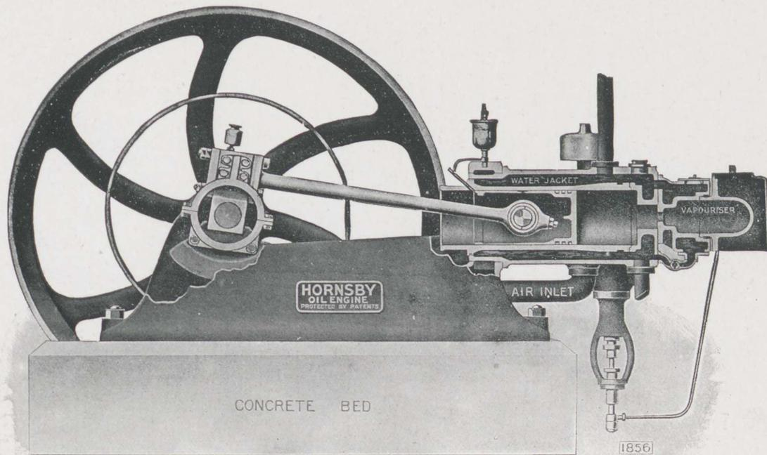
Fig. 131.—Section of Hornsby-Ackroyd Oil Engine
