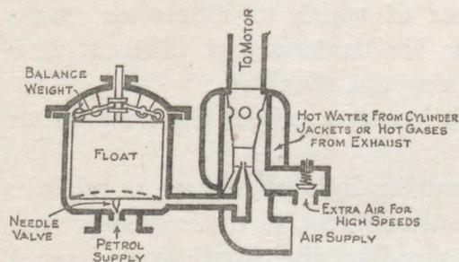
Fig. 117.—Diagrammatic section of a carburettor
