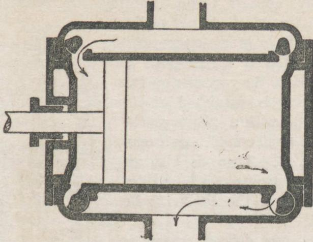
Fig. 76.—Diagram of a cylinder with Corliss valves
