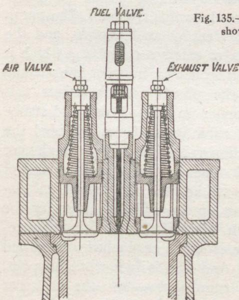
Fig. 136.—Section through cylinder cover
