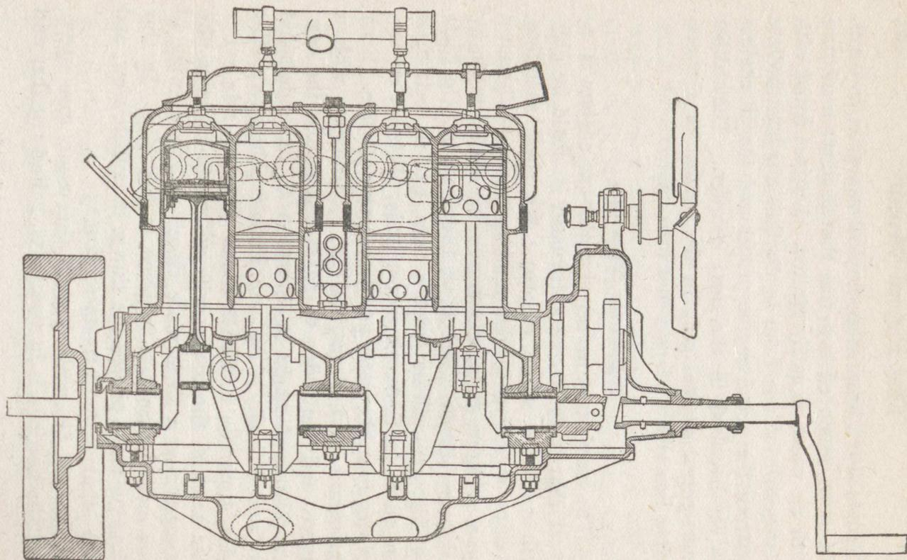
Fig. 123.—Longitudinal section of a 16-20 horse-power engine
