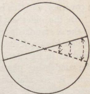
Fig. 157.—Diagram to illustrate torsion of a shaft
