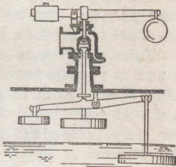
Fig. 46.—Safety valve with high and low-water floats
