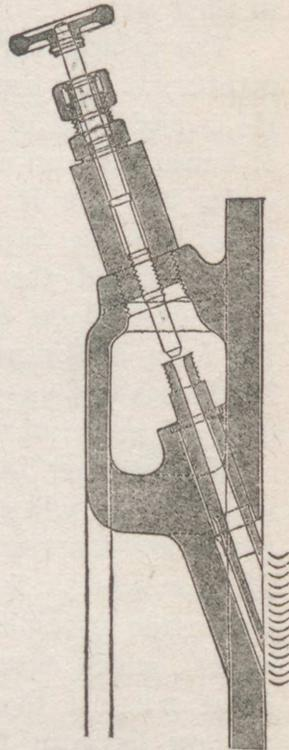
Fig. 87.—Section through nozzle of de Laval turbine
