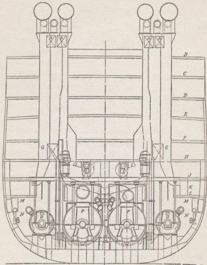
Fig. 172.—Section through turbine rooms of the *Aquitania*, looking aft
