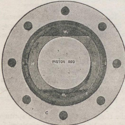
Fig. 62 (b).—Metallic packing; Transverse section
