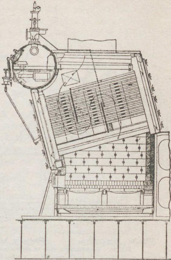
Fig. 42.—Section through Babcock and Wilcox marine boiler
