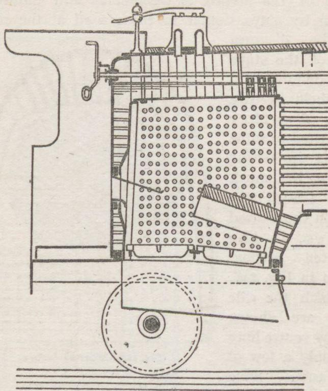
Fig. 149.—Typical firebox of British locomotive
