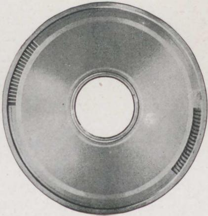
Fig. 95.—Diaphragm at high-pressure end
