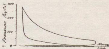
Fig. 178.—Indicator diagram of gas engine
