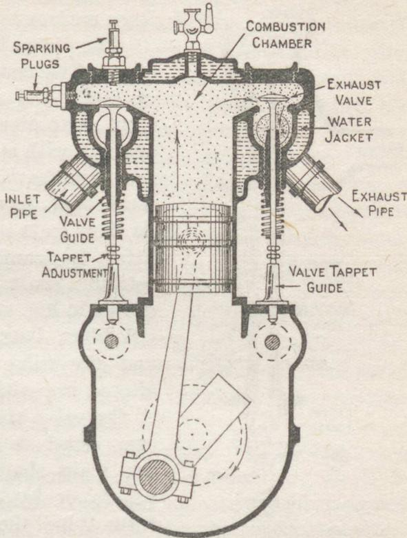
Fig. 118.—Diagram of petrol motor
