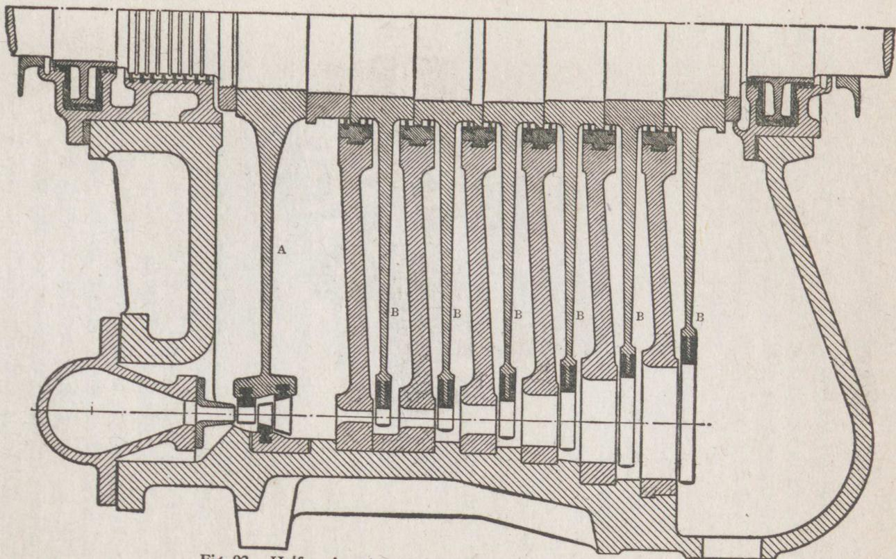
Fig. 92.—Half-section through large Westinghouse-Rateau turbine
