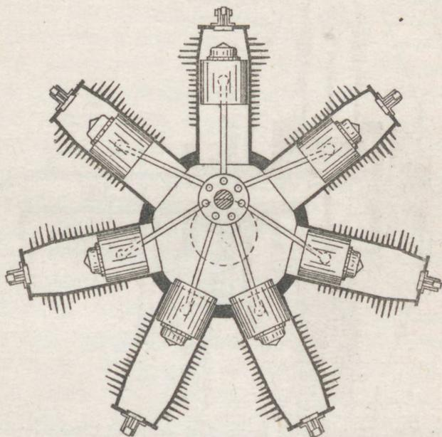
Fig. 128.—Diagrammatic transverse section of Gnome engine
