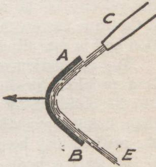
Fig. 88.—Diagram to explain principle of impulse turbine
