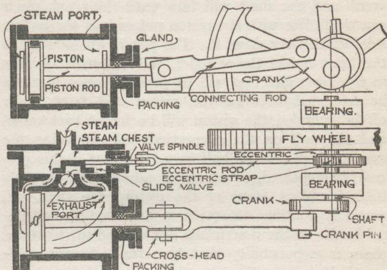
Fig. 6.—Diagram showing parts of a horizontal engine
