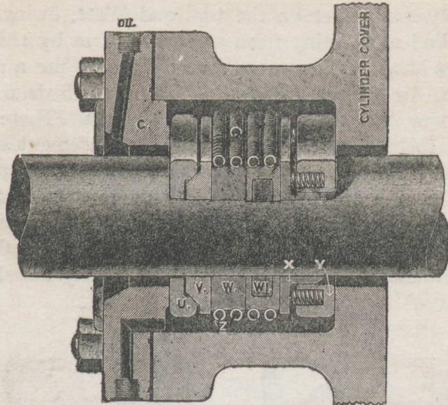
Fig. 62 (a).—Metallic packing; Longitudinal section
