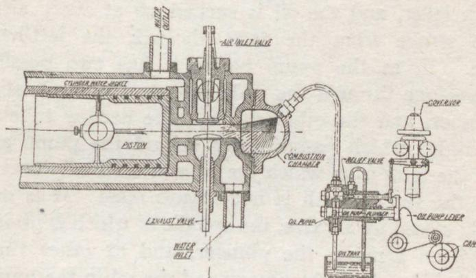
Fig. 140.—Section of Crossley semi-Diesel cylinder, vaporiser and oil pump
