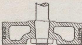
Fig. 59.—Piston for small engine
