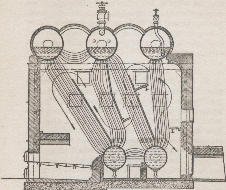
Fig. 38.—Interior of a Stirling boiler
