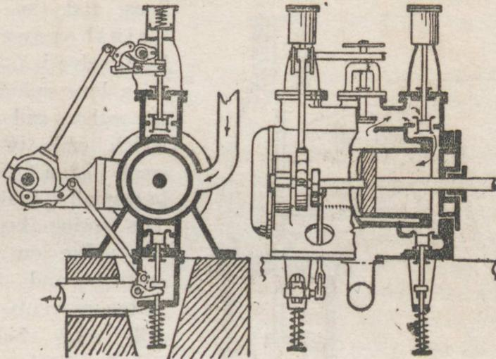
Fig. 78.—Transverse and longitudinal section through cylinder fitted with drop valves
