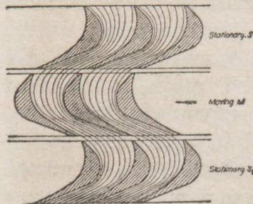
Fig. 90.—Diagram of blades of impulse turbine
