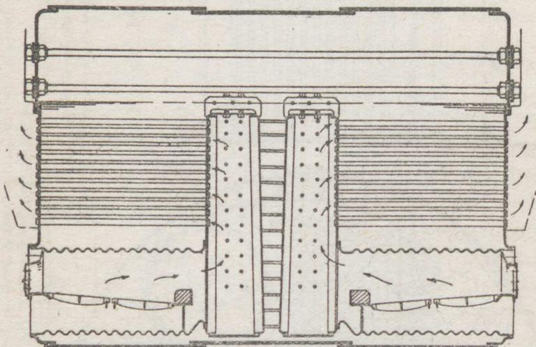
Fig. 36.—Double-ended marine boiler
