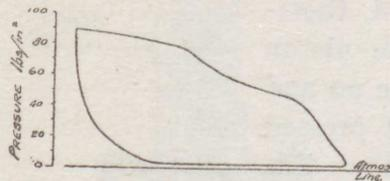
Fig. 177.—Indicator diagram of steam engine
