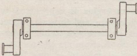
Fig. 66.—Crank for double-cylinder engine
