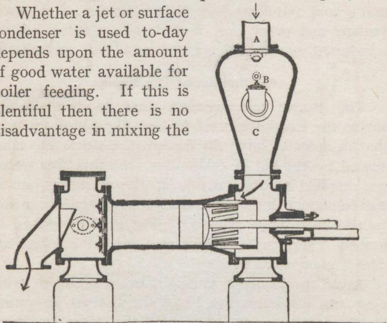
Fig. 84.—Combined jet condenser and air pump
