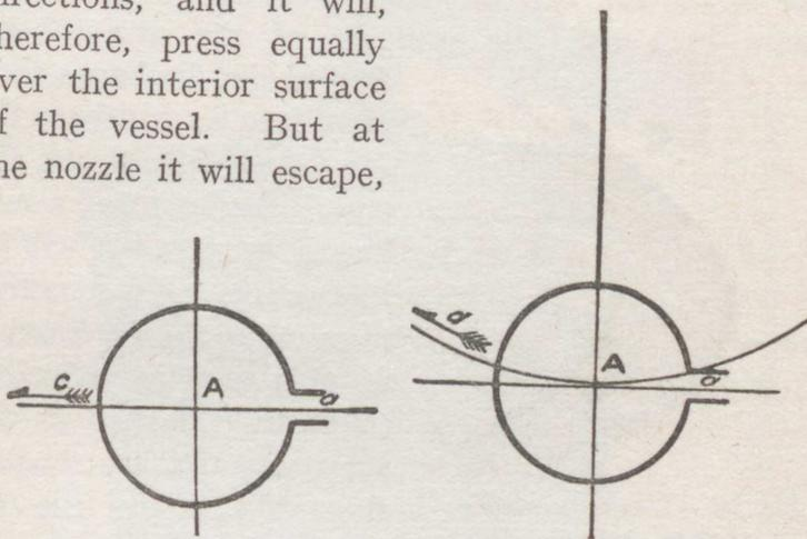
Fig. 100.—Diagram to explain reaction due to jet of escaping steam
