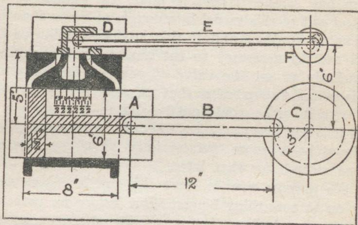
Fig. 11.—Model for study of valve motion
