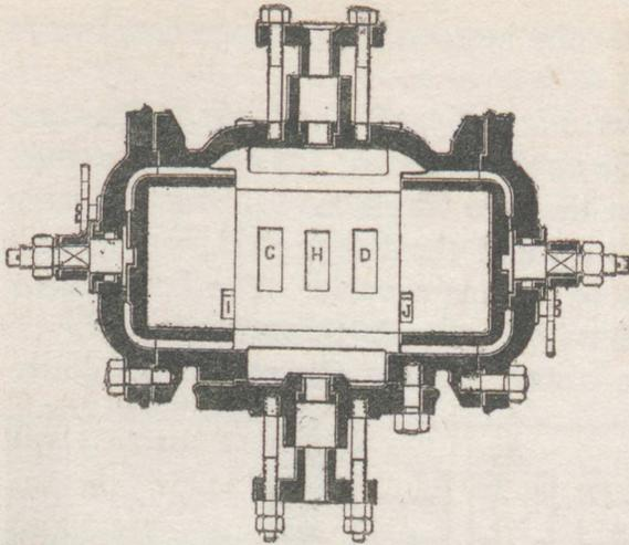
Fig. 162.—Ports through which steam enters or leaves cylinder of Weir pump
