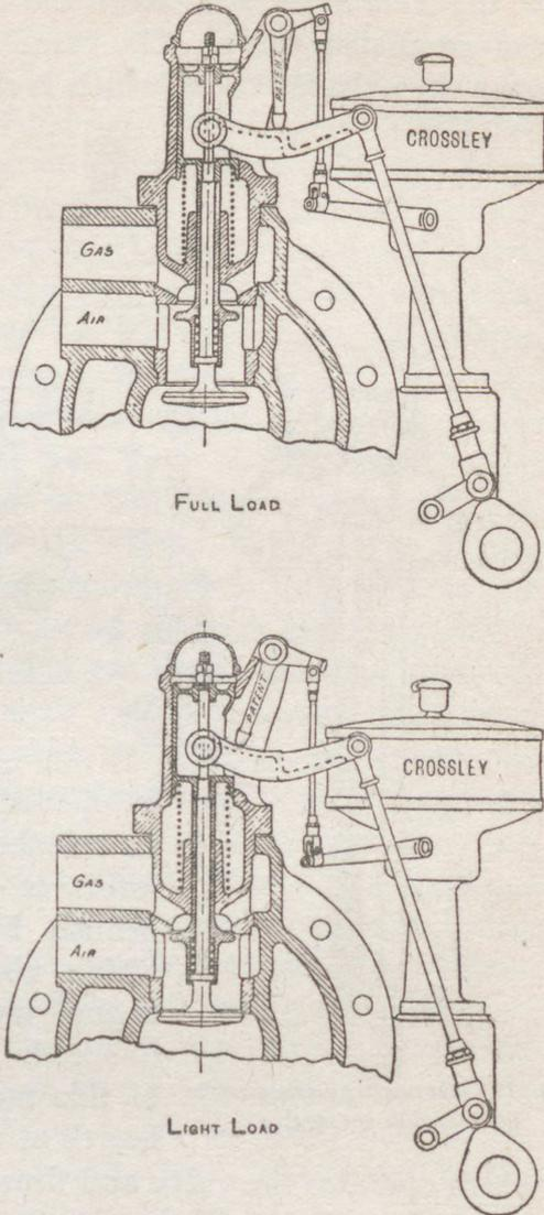
Fig. 112.—The governing arrangement of a Crossley gas engine
