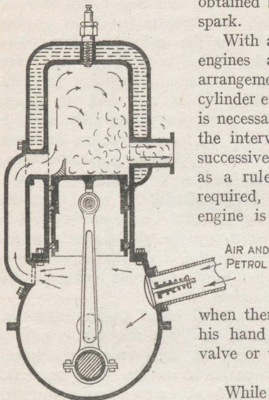
Fig. 120.—Diagram of two-stroke petrol motor
