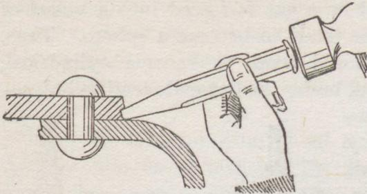
Fig. 23.—How the joints are caulked
