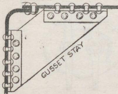
Fig. 22.—How the ends of a boiler are strengthened
