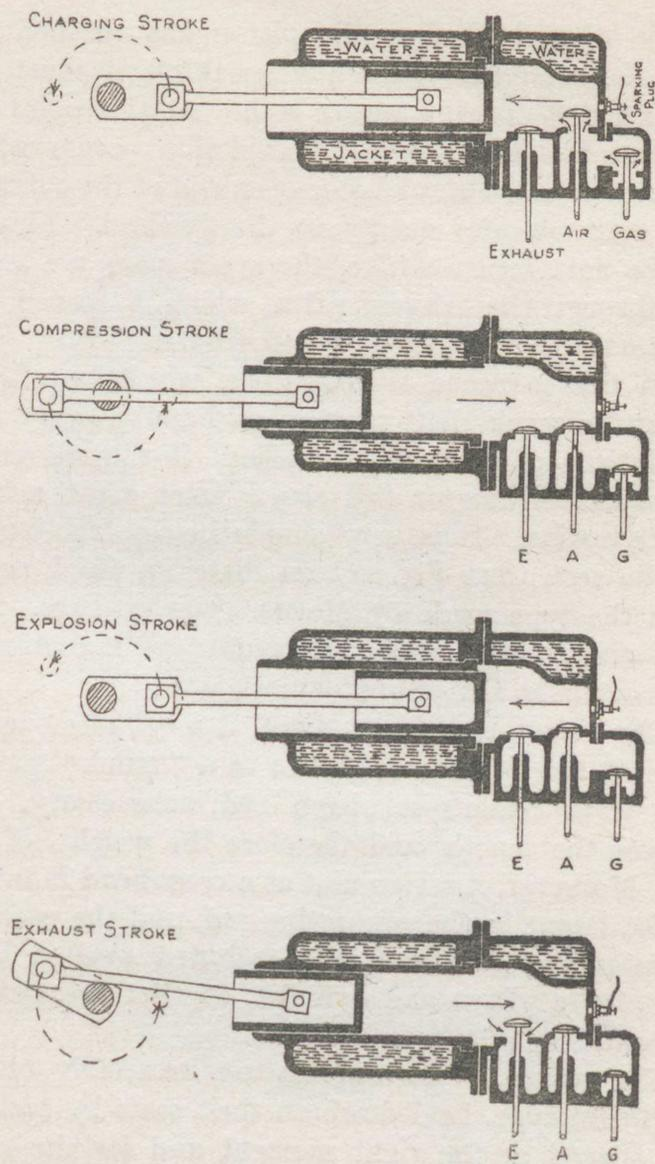
Fig. 110.—Diagram to explain how a gas engine works
