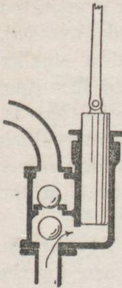
Fig. 55.—Simple feed pump
