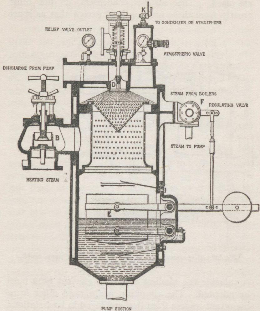
Fig. 160.—Weir's direct contact feed water heater
