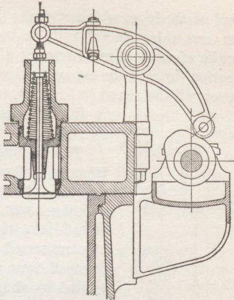
Fig. 135.—Section through valve showing jointed lever
