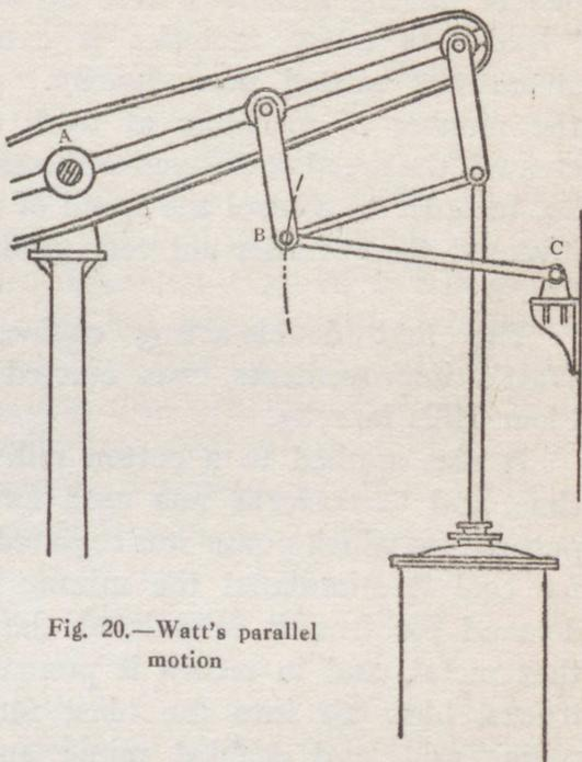
Fig. 20.—Watt's parallel motion
