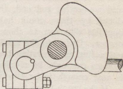
Fig. 64.—Balanced crank
