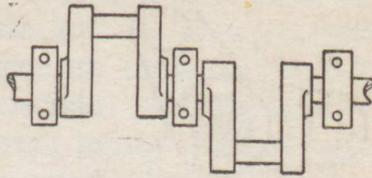
Fig. 65.—Crank for double-cylinder engine
