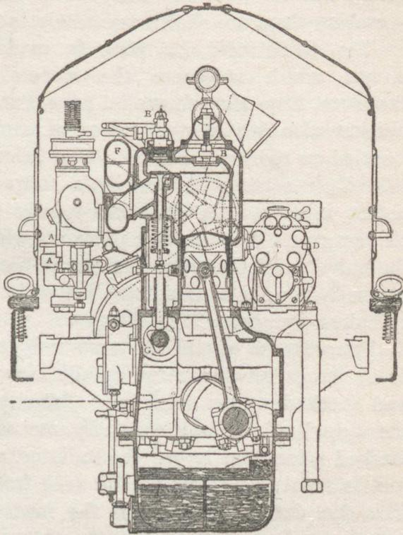
Fig. 124.—Transverse section of a 24-30 h.-p. engine
