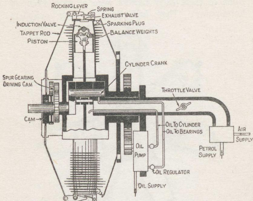
Fig. 129.—Diagrammatic longitudinal section of Gnome engine
