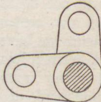
Fig. 67.—Two cranks at right angles
