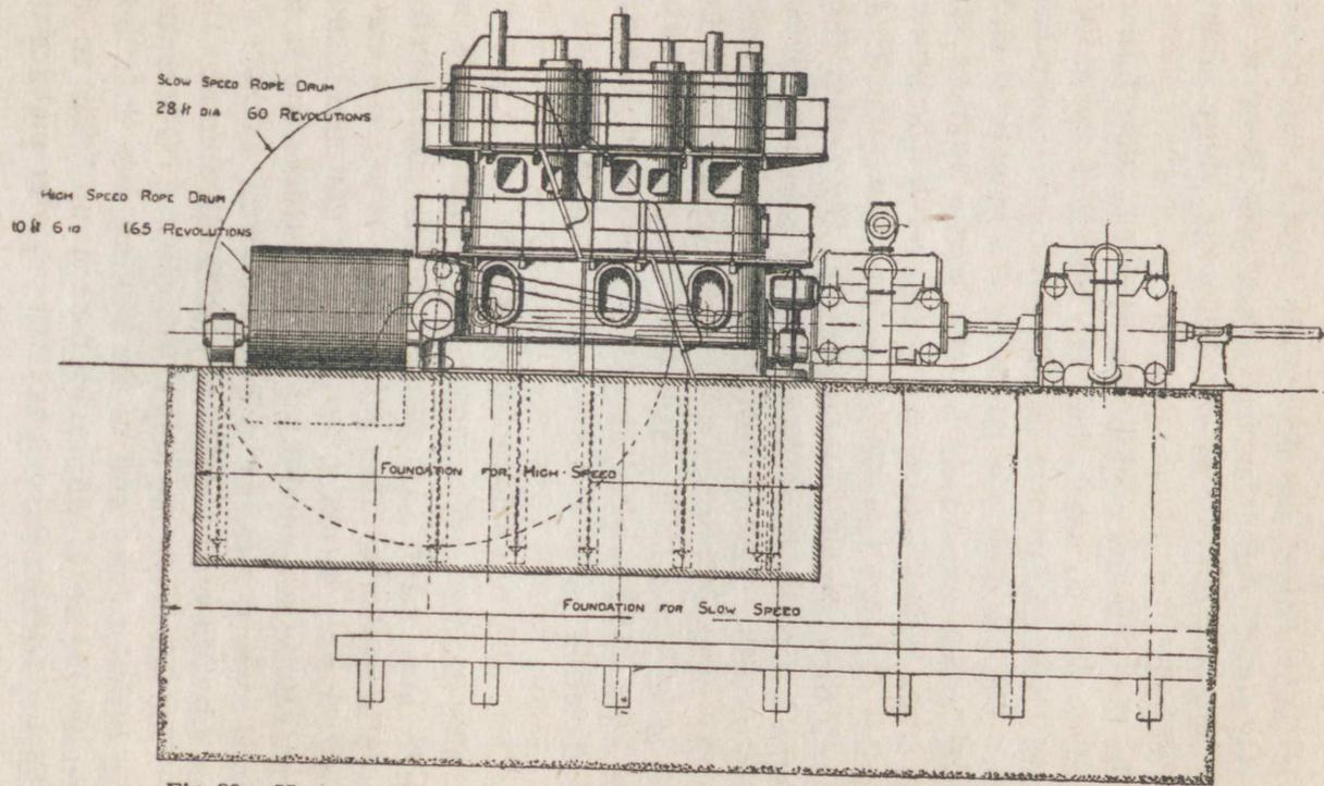
Fig. 80.—Horizontal and vertical engines of equal power drawn to same scale. Elevation
