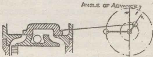
Fig. 10.—Slide valve with lap and lead
