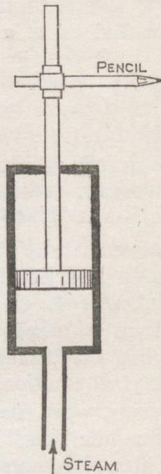
Fig. 175.—To illustrate principle of indicator
