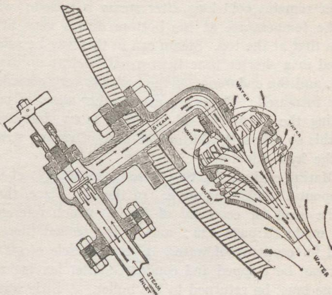
Fig. 158.—Weir's Hydrokineter
