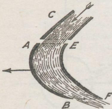
Fig. 101.—Diagram to explain principle of reaction turbine
