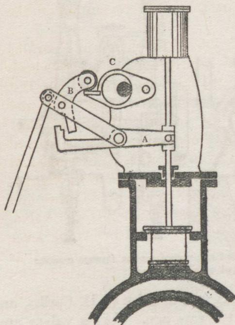
Fig. 79.—Mechanism of drop valve to larger scale
