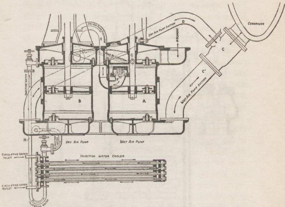
Fig. 159.—Diagrammatic section of Weir "Dual" air pump, cooler, and connections
