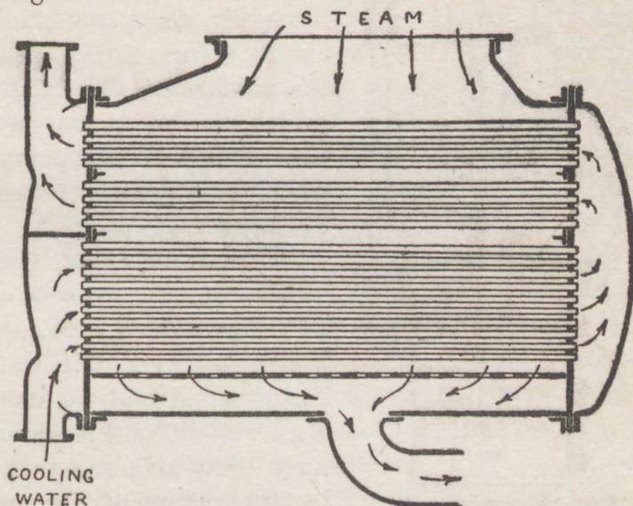
Fig. 85.—Section through surface condenser
