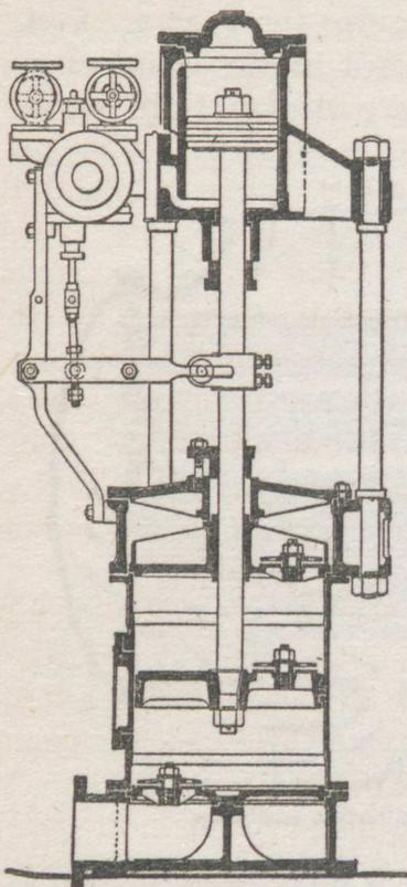
Fig. 86.—Section through Weir monotype air pump
