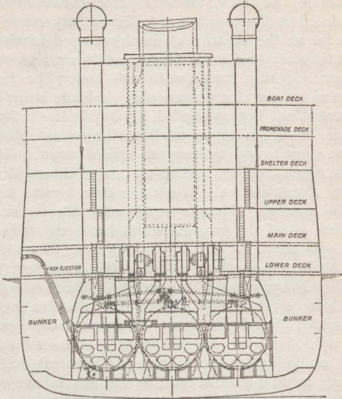
Fig. 170.—Section through boiler room of the *Mauretania*
