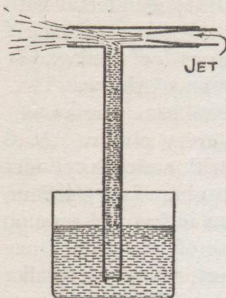
Fig. 57.—Principle of injector
