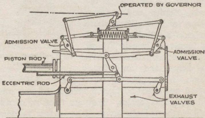
Fig. 77.—Corliss valve gear
