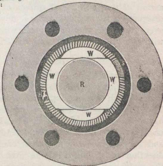
Fig. 63 (b).—Metallic packing for high pressures: Transverse section
