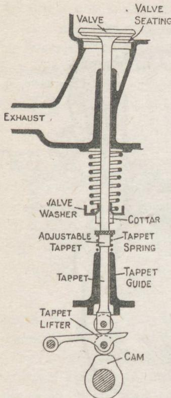
Fig. 119.—Adjustable valve tappet
