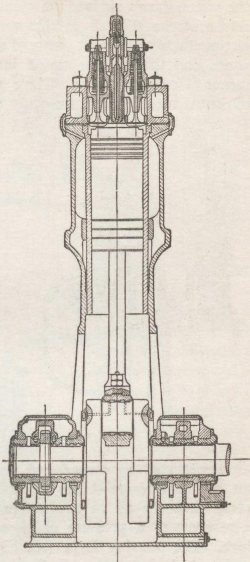
Fig. 133.—Longitudinal section of Diesel engine
