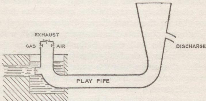
Fig. 116.—Diagrammatic section of the Humphrey pump
