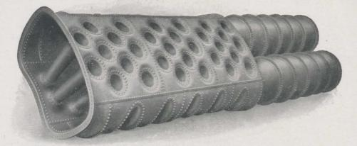
By permission of Messrs. Galloway, Ltd., Manchester Fig. 32.—Galloway's Flue
