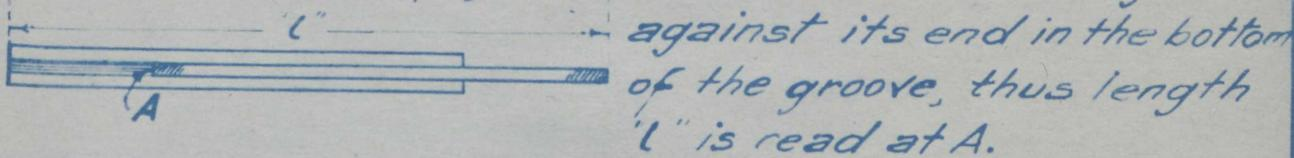
against its end in the bottom of the groove, thus length 'l' is read at A.
