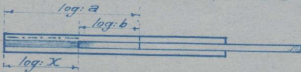
This sketch shows another way of division, but to set divider on slide against dividend on scale is troublesome unless dividend first is marked by the sliding index. This method is of use in combined multiplications and divisions when the index anyhow is in continuous use and where we are willing to take the errors that arise by using it.
