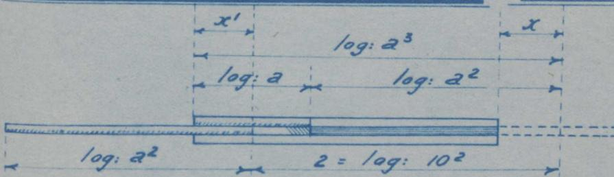
When higher numbers are to be cubed the slide can be reversed reading at  $x'$  instead of  $x$  outside the rule. It will be seen that the characteristic correction is 2.
